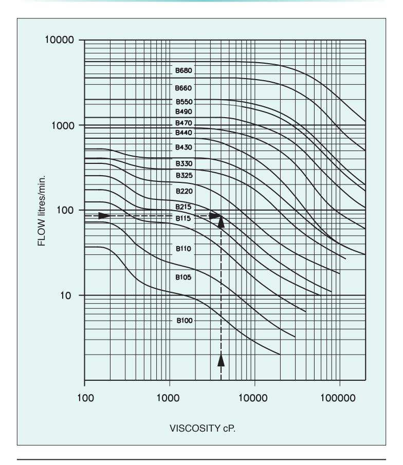
The curves on this chart define the fields of operation of the The appropriate pump is the model B 220. various sizes of pump, enabling a preliminary selection to be This preliminary selection should subsequently be checked on the made according to viscosity/flow.
