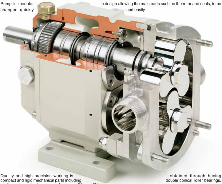
shafts and oversized gears running in an oil bath within the gearbox.
