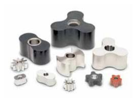
Dependant on the type of use the rotors can be made as: standard stainless steel tri-lobes, stainless steel bi-lobes, acteon dual wing rotary piston, gears for Models B100 and B105. The stainless steel tri-lobe rotors (5 lobes for Models B100 and B105) and stainless steel bi-lobes can all be covered with rubber in different compositions. The rotors are inter-changeable and should they need to be replaced it
