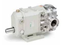
When the pump is transferring products that may crystallise or leave solid deposits, the mechanical seals supplied have to be cleaned by flushing water or a compatible liquid at low pressure. This flushing arrangement can also be used to dissipate heat or to avoid dry running. There is a fixed chamber around the standard seal with the UM seal for sealing the flushing liquid.
