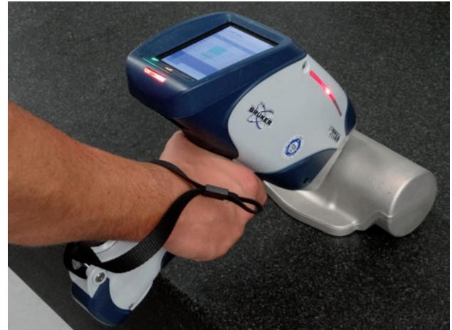
Spectrometer and RFA material analysis
