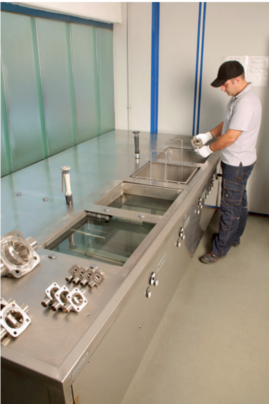
Ultrasonic cleaning of valve bodies
